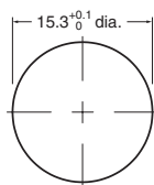
Panel Cutout Dimension Panel thickness = 1 to 4 mm
